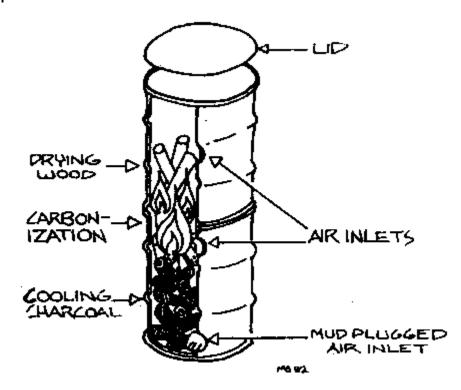
Attachment 9B: Basic principles of kiln design
